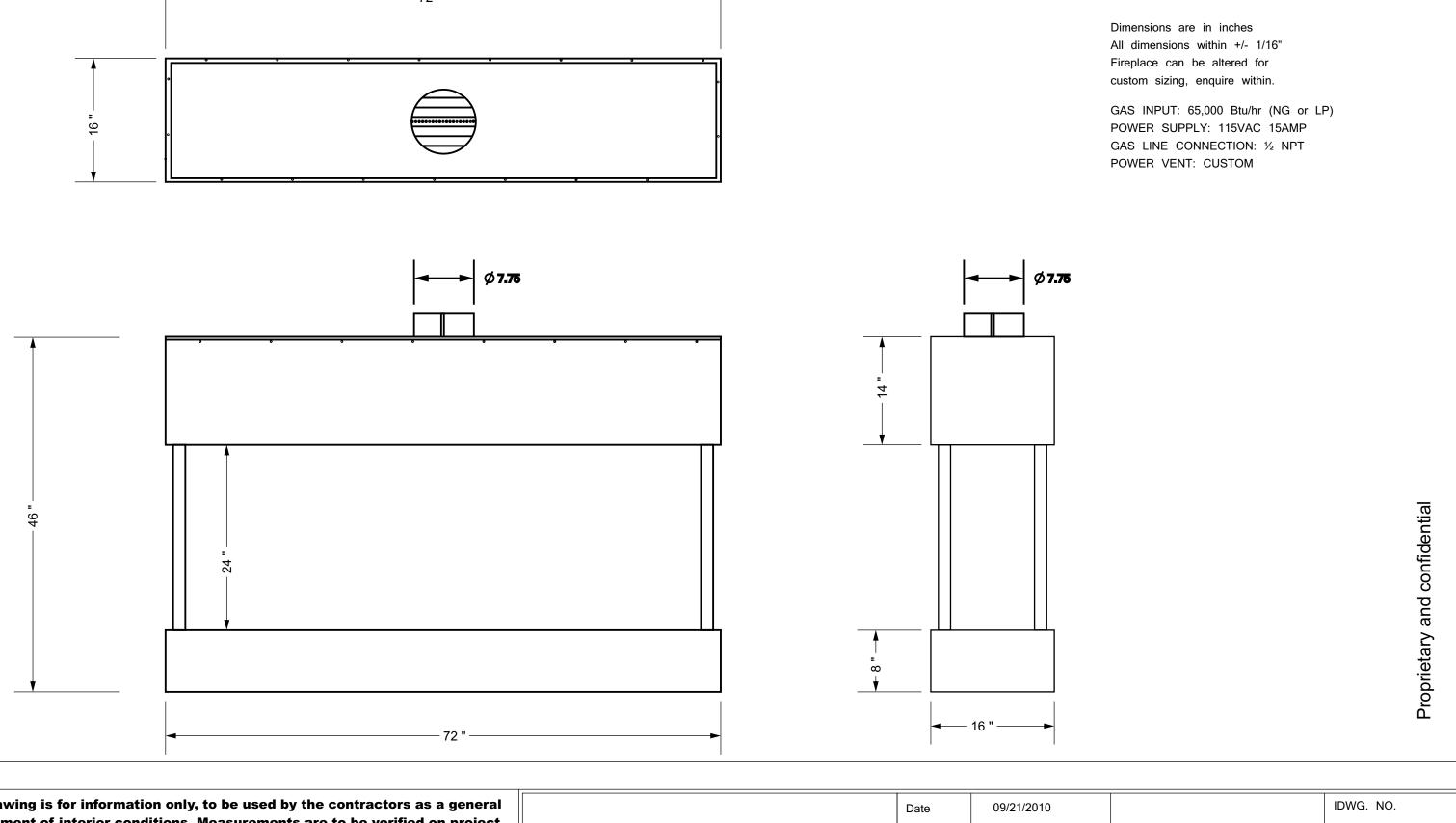
This drawing is for information only, to be used by the contractors as a general arrangement of interior conditions. Measurements are to be verified on project site, this drawing must be verified and approved prior to final detailing and fabrication. This drawing is the property of Fireplace Concepts North America and is not to be reproduced or copied in whole or in part. Any reproduction in part or as a whole without the written permission of Fireplace Concepts North America is prohibited.
